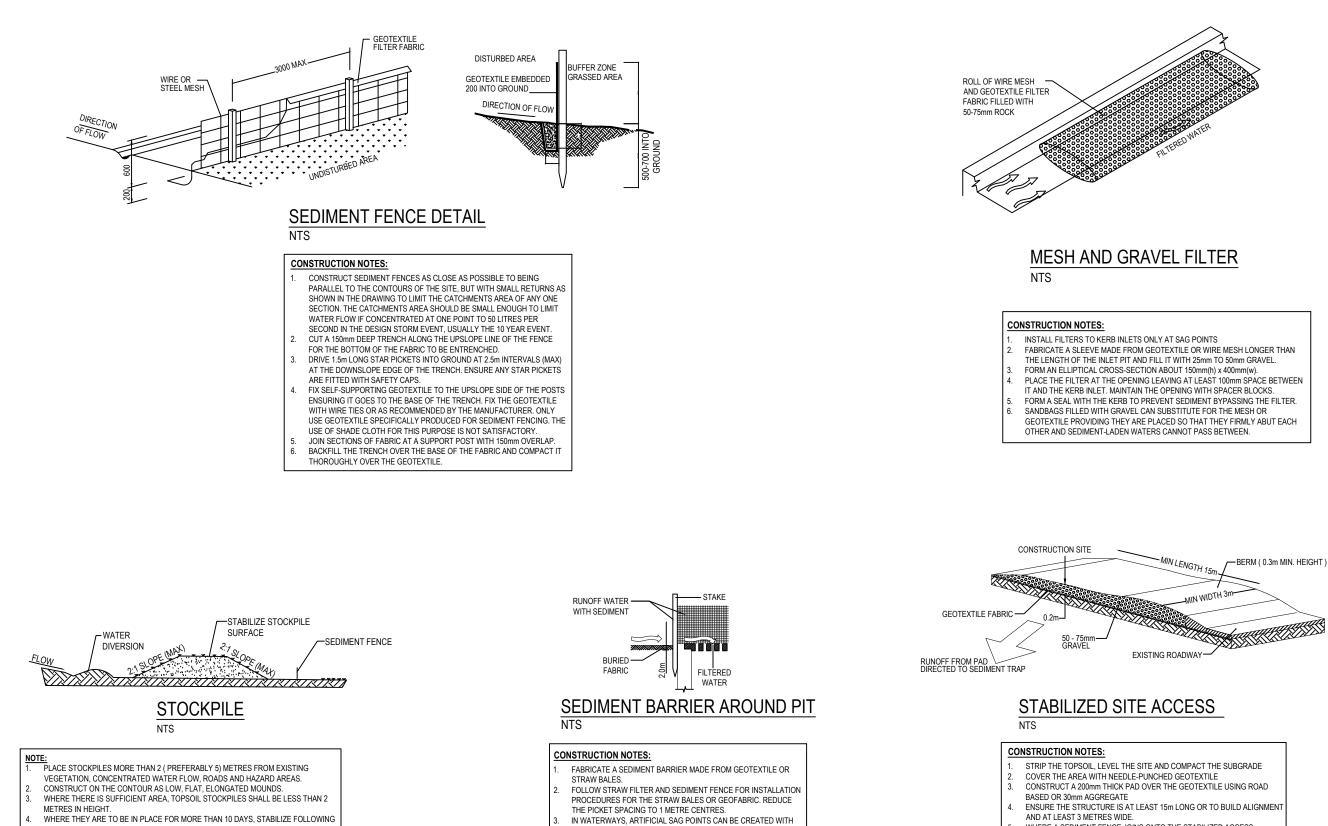
THE APPROVED ESCP OR SWMP TO REDUCE THE C-FACTOR TO LESS THAN 0.10. CONSTRUCT EARTH BANKS (LOW FLOW) ON THE UPSLOPE SIDE TO DIVERT WATER AROUND STOCKPILES AND SEDIMENT FENCES 1 TO 2 METRES ON THE DOWNSLOPE
